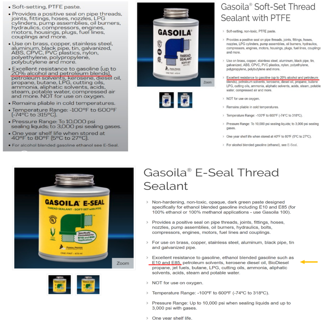
FIGURE 3. COMMON SEALANTS WITH MARKETED COMPATIBILITY FOR E15
