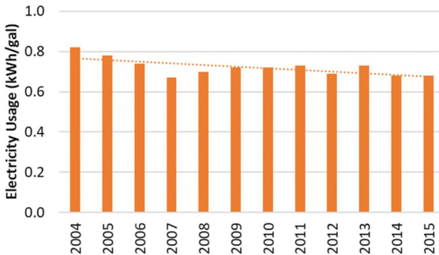
**Figure 5.5.** Electricity Consumption in Corn Ethanol. (ACE, 2018)
