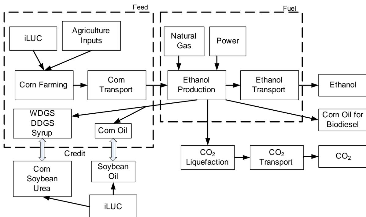
Figure 1.3. System Boundary Diagram for Corn Ethanol Production.
