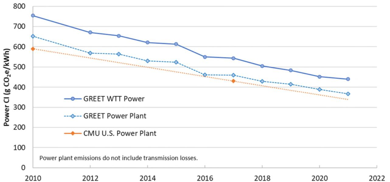
**Figure 6.2.** Carbon Intensity of Electric Power (U.S. Average).
