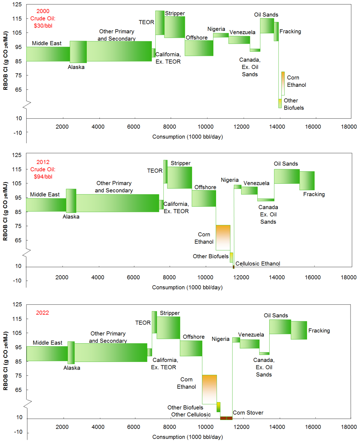
Figure 3.8. Carbon Intensity (g CO 2 e/MJ) of petroleum fuels versus consumption for the U.S.
